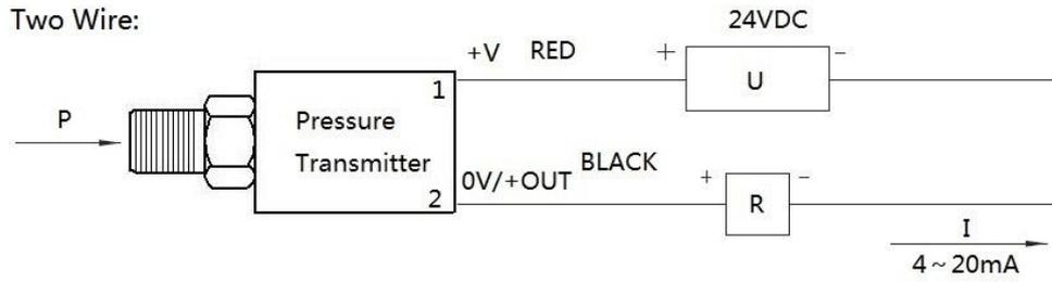
Two-wire 4 ~ 20mA current output electrical wiring diagram
